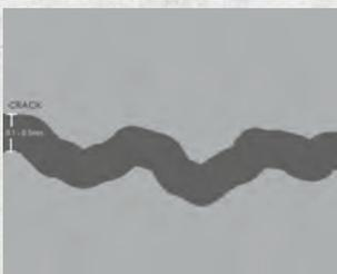
Concrete is porous and consists of microcracks, pores, and capillaries, which typically have a width between 0.1-0.5mm.
