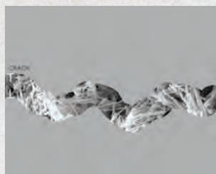
Water is unable to pass through the crystal formations and the concrete is now impermeable.
